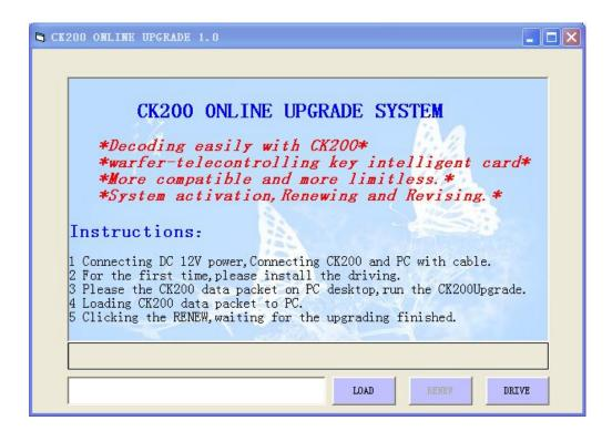
2. For the first time, click on the "DRIVE" button to install the CK200 drive.
