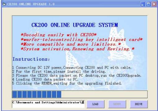
7.When the "ReNewing completed!Run?" dialog box appears, Click "Yes" to complete the upgrade.At the same time,The CK200 is in normal operationState. Then, you can remove the upgrade cable and the power adapter.
