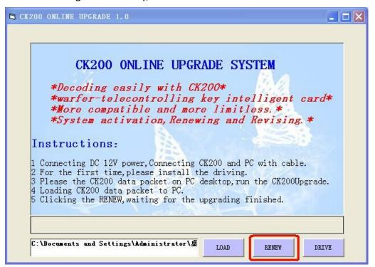
6.After Clicking the RENEW button"Upgrading, please wait....." will be showing on the CK200 screen. At the same time, a progressbar will be showing on the interface of CK200 client programe.
